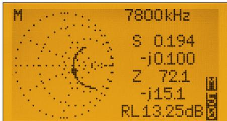
**Fig. 30:** Example of the multi-frequency measurement the reflection coefficient, the result is a small Smith chart; the real and Imaginary part and other calculated values are displayed below the marker frequency.
