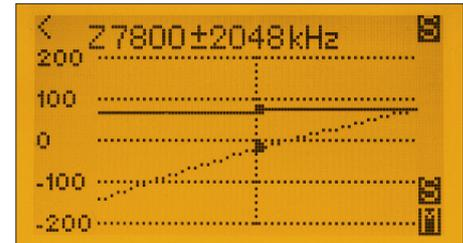
**Fig. 28:** Example of a multi-frequency measurement the impedance; using plus / minus buttons the centre frequency of the span area changes, as indicated by the arrow on the top left pointing towards the left side.
