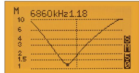
**Fig. 27:** Multi-frequency measurement of the SWR; The current marker values are displayed.
