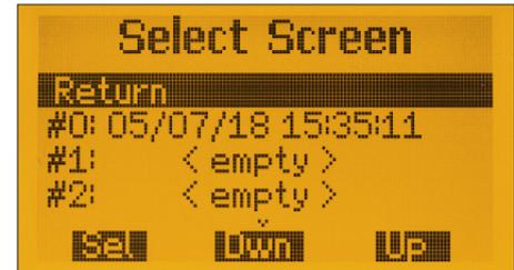
Fig. 37: A saved screen display with timestamp which can be re-called.
