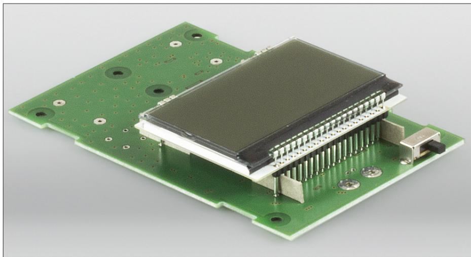
**Fig. 8:** Main PCB view before soldering the female connectors of the LC display; The cardboard strips must be pulled out after soldering, also the display is removed (unplugged) again before fitting the remaining components. 6-pin header for programming is obsolete
