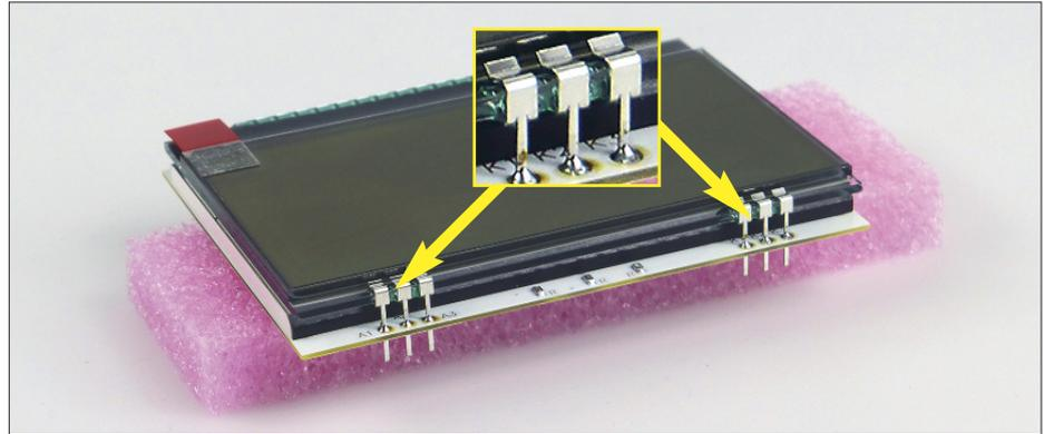
**Fig. 5: Display with backlight; all six connections must be soldered on top of the backlight PCB**
