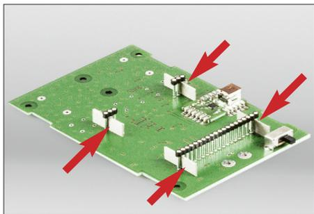
**Fig. 7:** Four cardboard strips are used for setting the distance between female connectors and the PCB.
