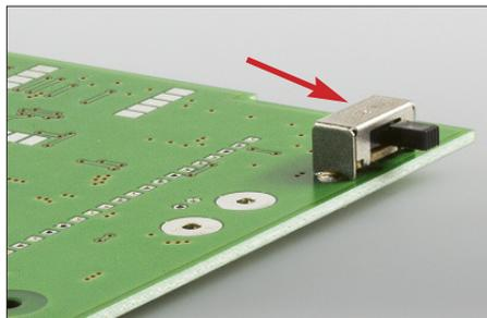
Fig. 3: Slide switch soldered in the correct position. 6-pin header is obsolete
