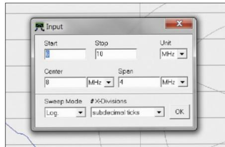
Fig. 64: Double-clicking on the corresponding Span label in Fig. 42 opens this input window for entering the start and stop frequency
