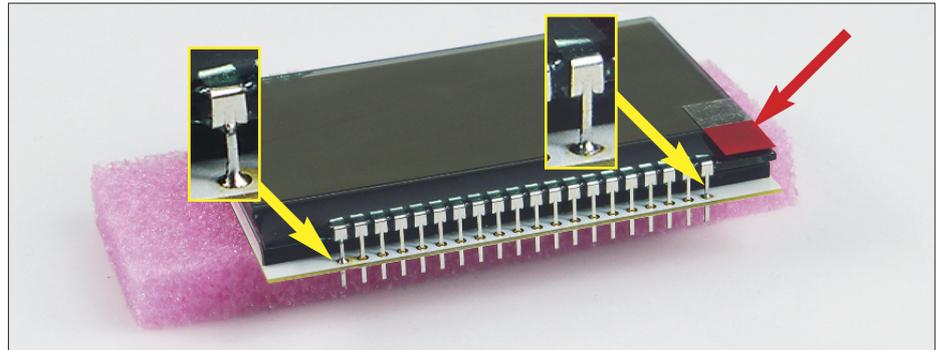
**Fig. 6: View of the 20-pin contact strip of the display after assembly. Only the two outer pins are soldered on top of the backlight PCB. Remove the protective film from the display by pulling the red tab.**
