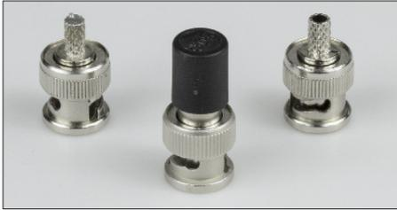
**Fig. 12:** The kit contains a set of calibration elements for use in the frequency range up to about 100 MHz, consisting of a 50 Ω Termination from *Telegärtner* (centre) and two BNC coaxial cable connector for making the Short and Open reference elements (see text).
