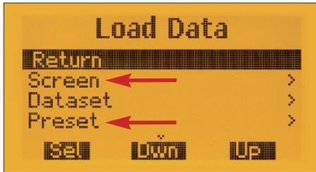
Fig. 35: Access to saved Screens and Presets
