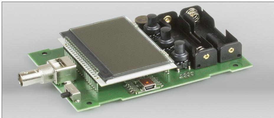
**Fig. 9: FA-VA5 Main Printed Circuit Board: fully assembled (6-pin header is obsolete)**
