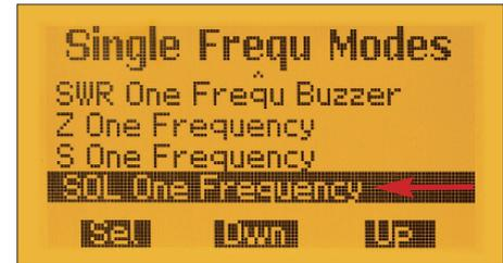
**Fig. 13:** Menu item for SOL compensation for the actual frequency
