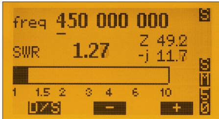
Fig. 20: Single frequency measurement SWR
