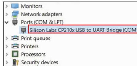
**Fig. 55:** Section from the display of the Windows Device Manager showing COM port used by FA-VA5 in USB mode.
