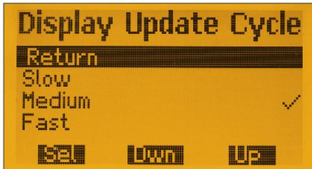
Fig. 46: The display repetition rate can be set to *Slow*, *Medium* or *Fast*.
