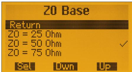
Fig. 49: Selection options for the Reference impedance basis
