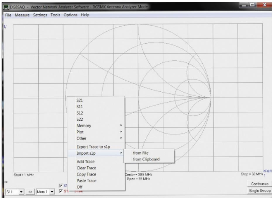
**Fig. 61: Selection menu for transferring data from a file or from Windows clipboard into the measured value memory of VNWA**
