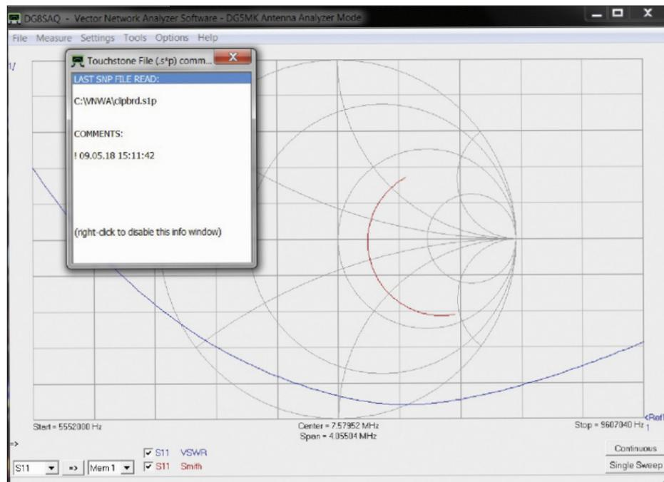
**Fig. 62:** Main window after importing a data set from the clipboard to the S11-measurement trace
