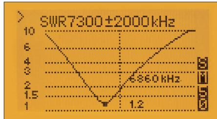
**Fig. 26:** Multi-frequency measurement of the SWR; the arrow on the top left, pointing to the right shows that an increase or reduction of the frequency span range can be made using the plus or minus buttons.
