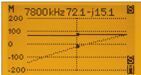
**Fig. 29:** Example of the multi-frequency measurement the impedance; the real and imaginary parts are displayed next to the marker frequency.
