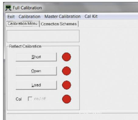
Fig. 65: Calibration window of the VNWA software prior to the start of the calibration process
