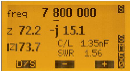
Fig. 21: Single frequency measurement of Impedance
