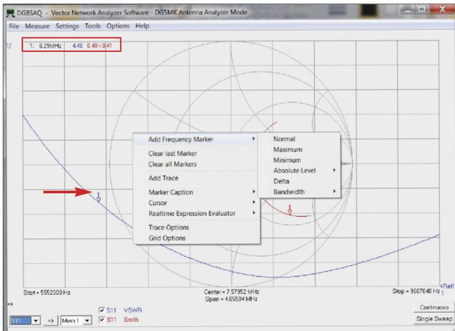
**Fig. 63:** Context menu when adding a frequency marker; the data of marker 1 (Arrow) can be seen in the upper left corner of the diagram (framed in red).
