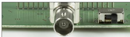
**Fig. 10: Slide switch in position Off**
