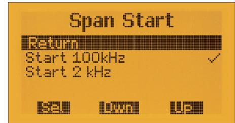
Fig. 53: Selection of the Sweep increment/decrement options of the frequency span for multi-frequency measurements
