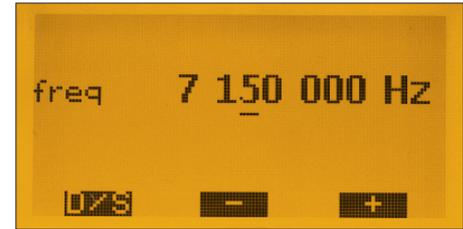
Fig. 31: Screen display when operating the FA-VA5 as an RF generator
