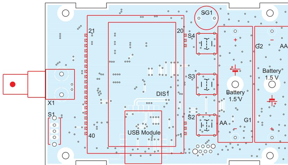
Fig. 2: Assembly plan of the FA-VA5 with components to be fitted
