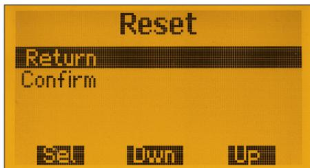
**Fig. 54:** This menu allows reset to the factory settings.
