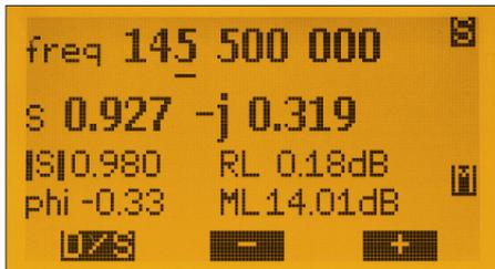
Fig. 22: Single frequency measurement of the Reflection coefficient
