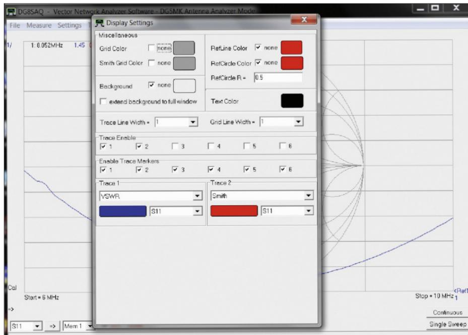
**Fig. 67:** The menu *Display Setup* offers a high degree of flexibility in the selection of the displayed measurement results; here only two traces are activated.
