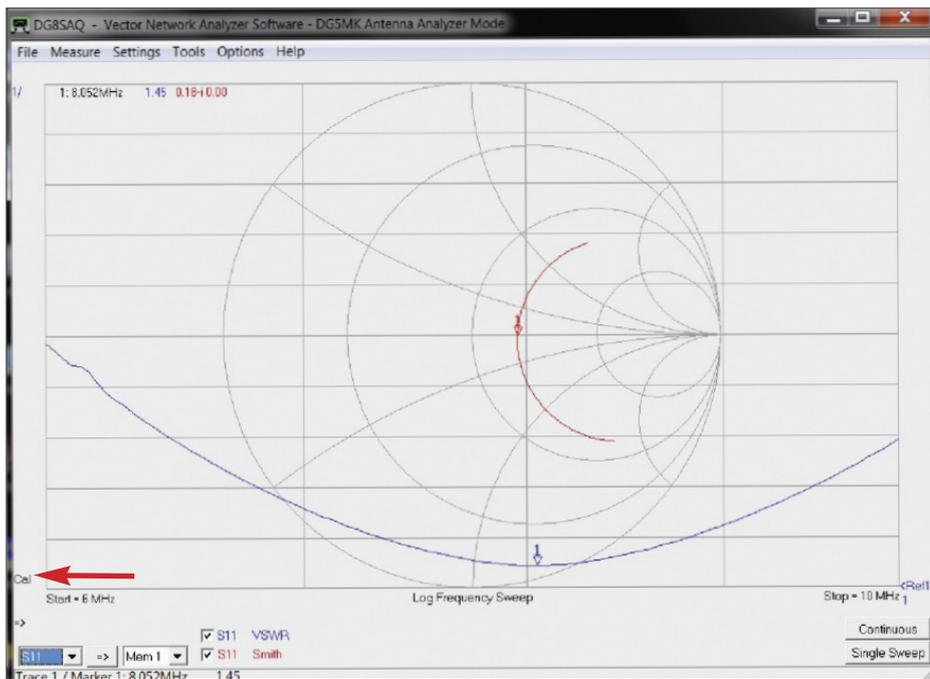
**Fig. 66: Result of a measurement run after calibration (arrow).**
